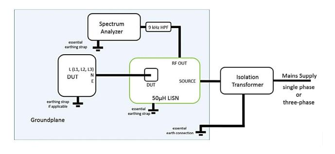
Figure 3 – Conducted noise pre-compliance measurement setup
