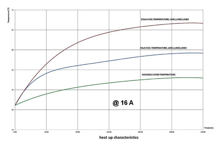
Figure 103: Coil and housing temperature at 16 A DUT current @ 22 °C ambient temperature
