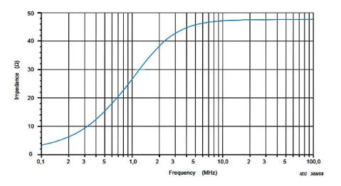
Figure E.1 - Characteristics of the AN impedance
