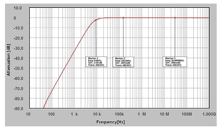
TBHPF1-9kHz: Attenuation 10 Hz to 1 GHz, typical data
