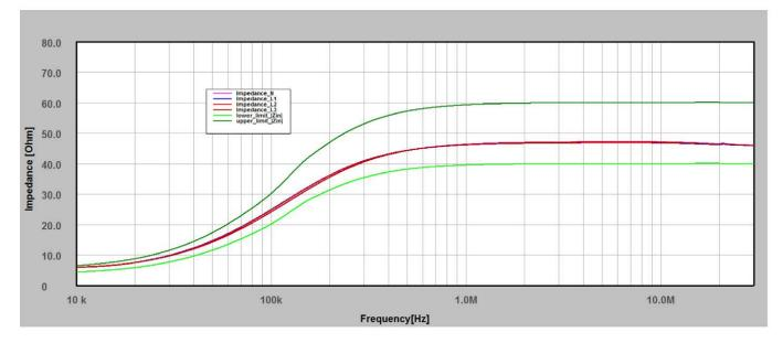
\*) BNC connectors terminated with 50 Ohm. Impedance measured at the DUT terminals on the PCB. The wiring from DUT connector to the PCB can be considered as an additional 20 cm of DUT supply cable length.
