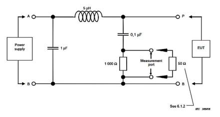
Figure E.2 - Example of 5 µH AN schematic
