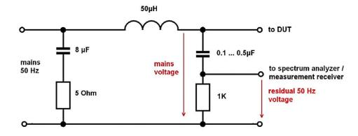
The full AC mains voltage is present at the DUT terminals of the LISN. The RF coupling capacitor and the 1K resistor form a voltage divider, which determines the amplitude of the 50 Hz voltage at the RF connector.
