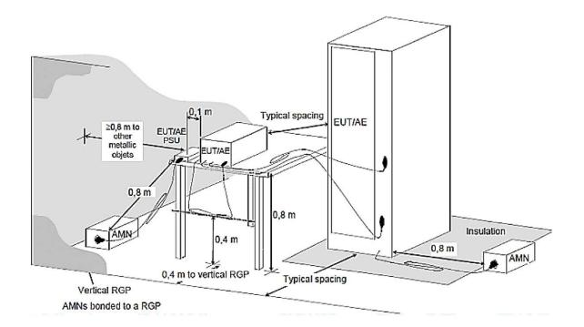
Set up for combination equipment
