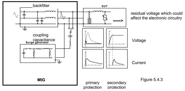
Superimposing SURGE pulses onto power lines is carried out using a capacitance between the tester and the power line. With the SURGE test, the effectiveness of the protection circuit will be tested. The residual voltage after the protection circuit could affect the electronic parts of the EUT.
