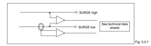
For the damped oscillatory tester the output at no load is calibrated to the charging voltage. Charging voltage are equal the output voltage at open circuit.
