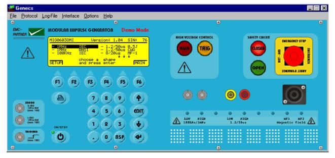
The GENECS windows is equal the MIG tester front plate. Online the MIG tester can be remote controlled by pressing the buttons with the mouse cursor as on the real front plate.
