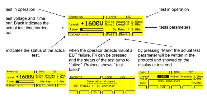
When a printer is connected to the MIG tester or the MIG is controlled from a PC with GENECS the following protocol will be printed or showed on the monitor:
