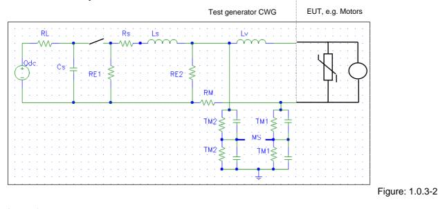
Legend: RL Charging resistor Cs Impulse capacitor High voltage switch S Serial resistor RF1 Discharge resistor Inductance of the generator Rs 1s RM Shunt RE2 Discharge resistor TM1 Divider Inductance of the connection MS Measurement equipment TM2 Divider Lv
