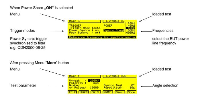
At Synchro =ON, the surges are released synchronous to the main frequency of an external coupling filter e.g. CDN2000-06-25
