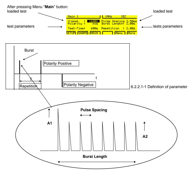
With pulse spacing the repetition frequency of the 1MHz or 100 kHz can be selected 1/tperiode = frequency. e.g. 400 Hz = 2.5 ms pulse spacing
