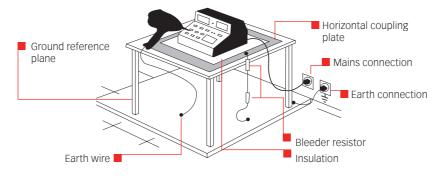
Example of a simplified test rig for a table-top instrument.
