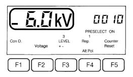
The instrument switches over from positive to negative polarity once half of the preset number of pulses has been released (the sign on the display changes).
