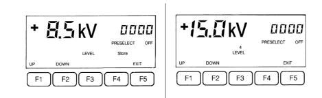
Press F5 to return to the starting menu level. (This return will also be made automatically after about 10 s).
