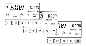
F5 sets the counter either back to 0000 or to the preset value if the preselect counter mode has been chosen.
