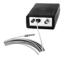
The normal remote trigger unit consists of a «triggerbox» and 5 m (197 ") of optical cable. The remote trigger works in parallel with the «trigger-button» on the NSG 435. Pulse triggering, or the on/off switching in the case of repetitive discharges, can be effected by a push-button or an electrical signal applied to the triggerbox.
