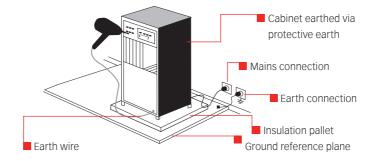
Example of a test rig for a system.
