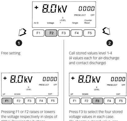
100 V. Pressing the buttons continuously changes the voltage level with increasing rapidity.
