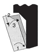
Insert the lower end of the battery (the part with the spring-blade) into the handgrip. Gently pull down against the spring so that the battery can be snapped inwards and then release the pressure.
