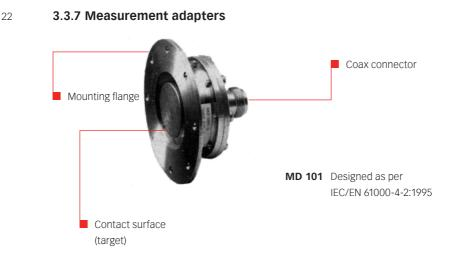
The measurement adapter type MD 101 as per informative annex B of IEC/EN 61000-4-2 serves to verify pulse amplitudes and pulse shapes. It is designed for mounting in the side wall of a Faraday cage in which an oscilloscope has been installed. This measurement adapter, also known as a «Pellegrini-Target» has the flat impedance curve to well over 1 GHz that is necessary for the purpose.
