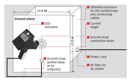
Teseq uses the following instruments for calibration purposes:
